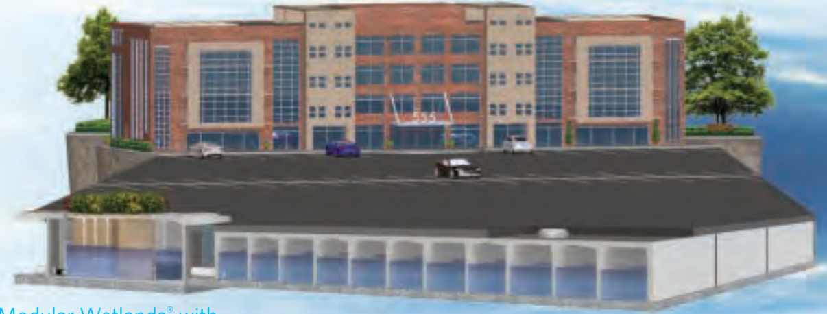
Modular Wetlands® with Box Culvert Prestorage
