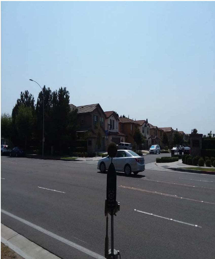
NM3 looking SW across S Western Avenue towards Donovan Ranch Road intrsection . A total of 203 vehicles passed the microphone travelling along S Western Avenue during 10 minute noise measurement.
